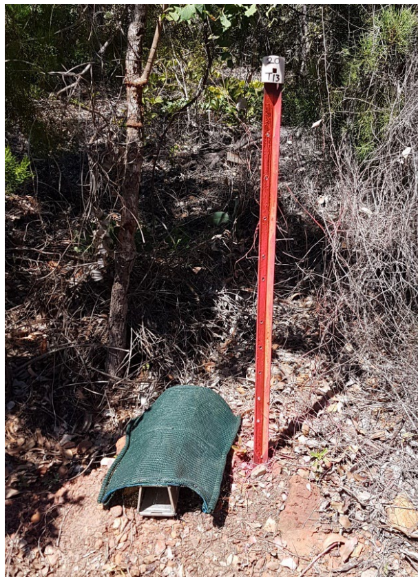
Plate 7-1: Example: Elliot trap covered by shade cover, marked with a labelled survey peg
